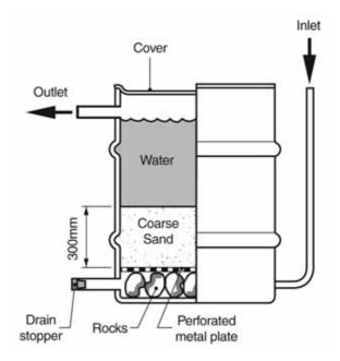
The sand will do most of the filtering of the small organism and microbes and the rocks are just there to hold the plate and sand and allow the filtered water to perculate up and be caught at the top.
